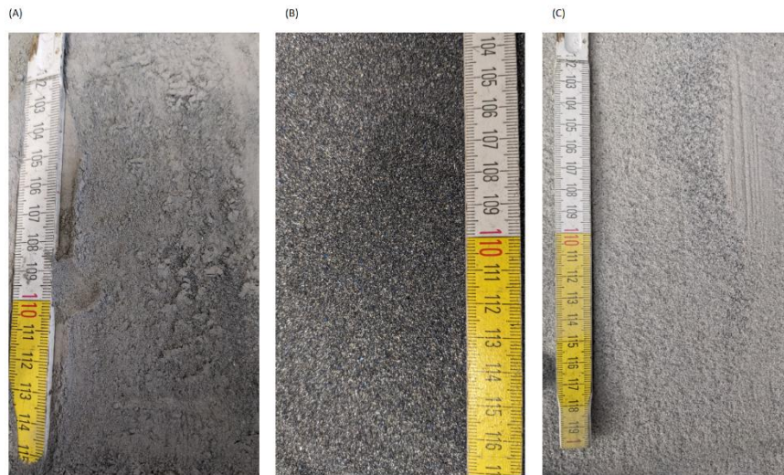
Figure 5 Black mass PV shred material, provided by Fraunhofer containing varying amounts of Si, Cu (0.9 %), Ag (2.6 %), Pb (0.3 %), Sn (0.6 %), Al etc.
